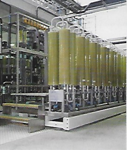
Left: Three parallel 70,000 gpd RO leachate treatment skids; right: 25,000-gcd containerized RO leachate treatment system
